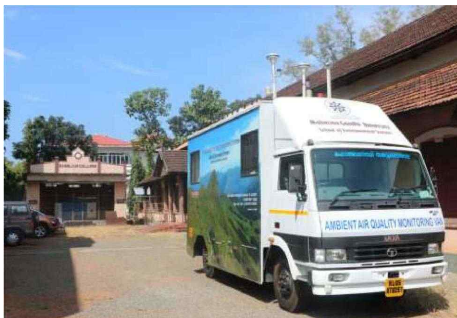
Fig. 4.1 Mobile ambient air quality monitoring van
